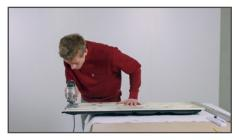
Saw, e.g. with a circular saw with a guide rail, slowly along the marking. If necessary, cut notches with a jigsaw.
